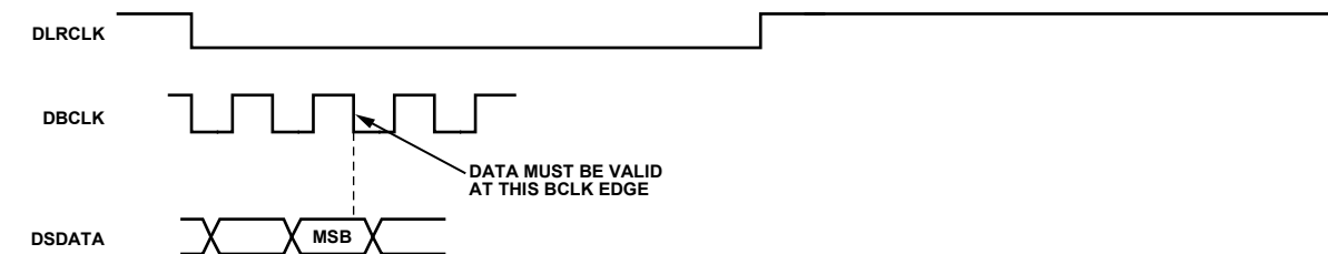
Figure 28. I 2 S Pipeline Mode in DAC Serial Data Transmission (Applicable in Stereo and TDM Useful for High Frequency TDM Transmission. This Model Is Also Available in the ADC Serial Data Port.)
